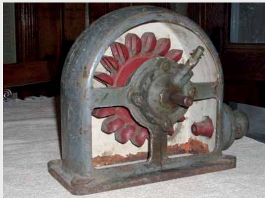
A late nineteenth-century water motor with one side of the casing removed. (www.oldpelton.net)
